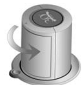
Rotate speaker counter-clockwise to return to the initial raised position in order to lower speaker.
